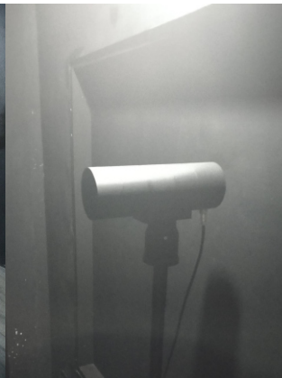
GONIO PHOTOMETRIC AND CCT TEST
