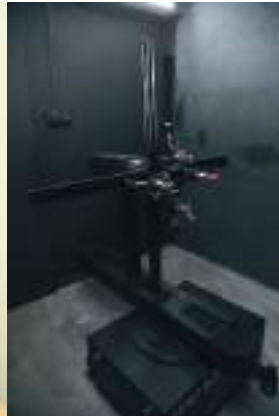
GONIO PHOTOMETRIC AND CCT TEST
